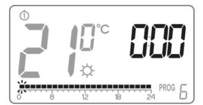
Blinking rectangle indicates the point of the timeline which is modified.
