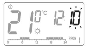
4. A flashing symbol of the day of the week appears in the upper left corner. Turn the knob to the left or right to set the day and confirm the selection using the (or) button.
