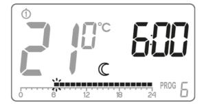
6. By pressing the selecting time interval the entire program is modified.
